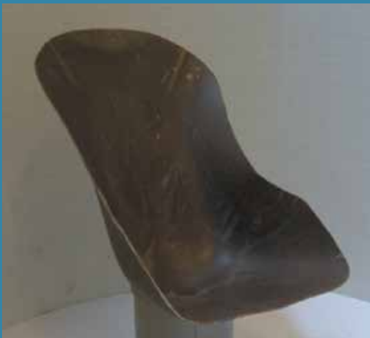
Prototype bio-based composite car seat
