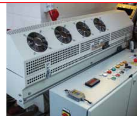
Image: Apparatus developed by Centexbel for the evaluation of the laser protection
